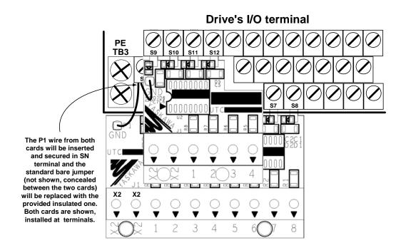
Figure 2. Installing both UTC000100 and UTC000120 on the G7 to cover all 12 digital inputs, S1 thru S12.
